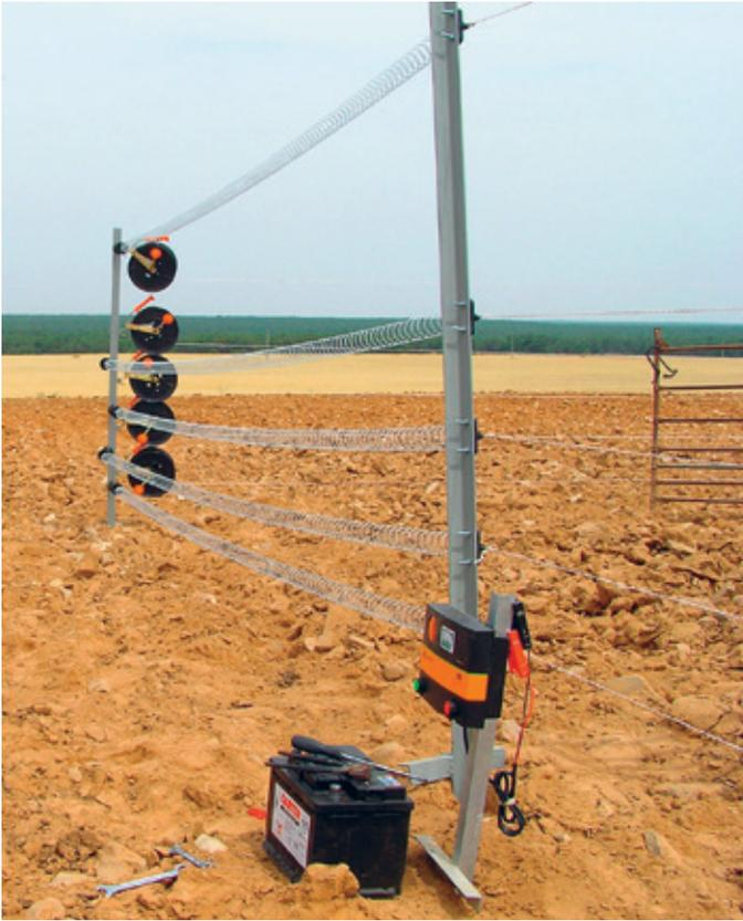
Mobile electric fences can be transported and installed by a single person in a short time.
